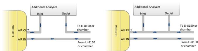
**Figure 1.** Plumbing schemes for connecting an additional analyzer in to the LI-8100A System. Left hand panel: series configuration. Right hand panel: parallel configuration.
