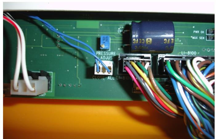
**Figure 2.** Pressure Adjust potentiometer.
